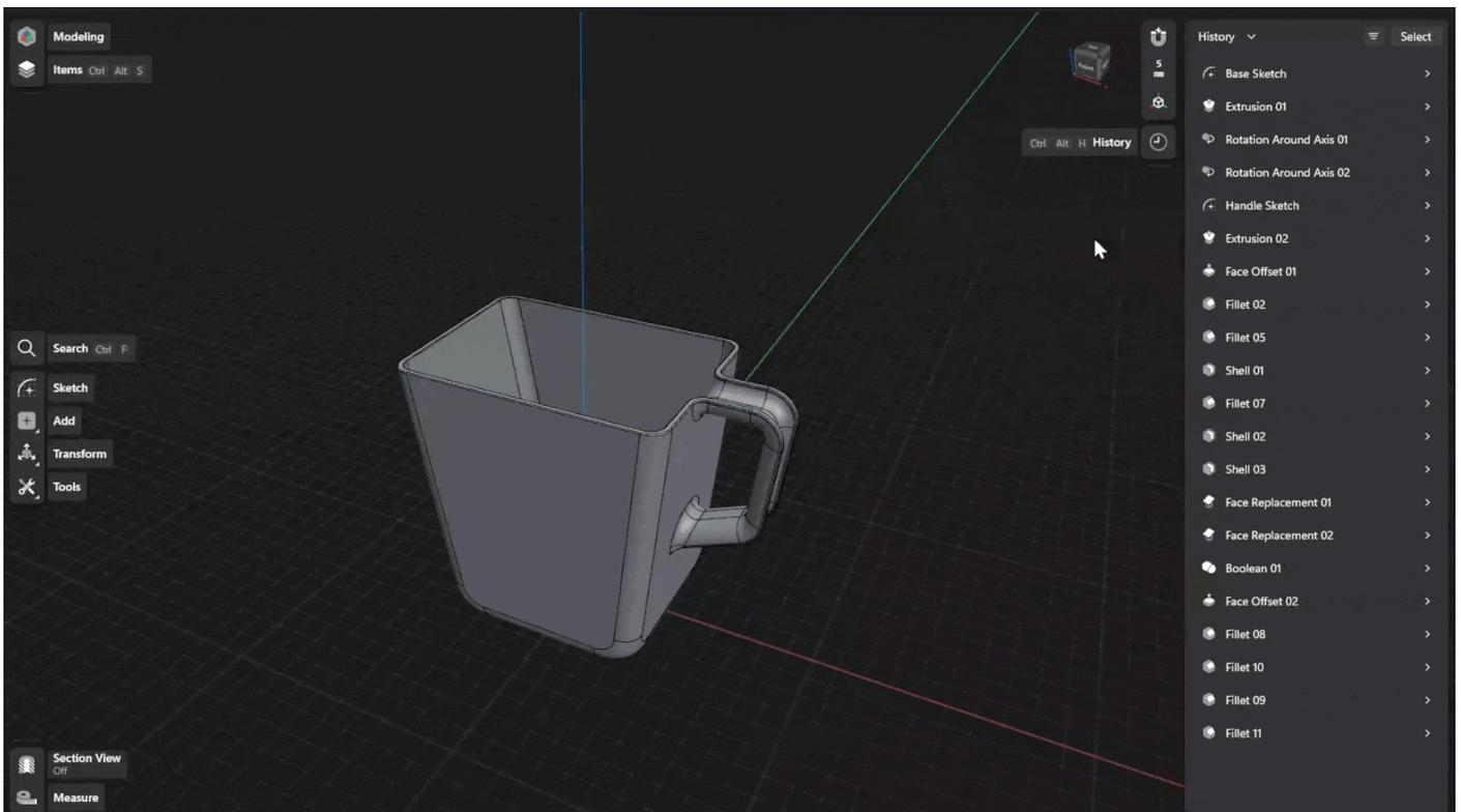
By removing the **Base Sketch** step, we eliminate the reference of all the succeeding steps, causing each step in the design history to break, and the model to disappear as shown by the yellow warning labels.
