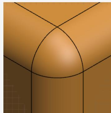
**Setback** This type of corner sets back the edges where the fillets begin blending into the corner. The blended face has a variable radius.
