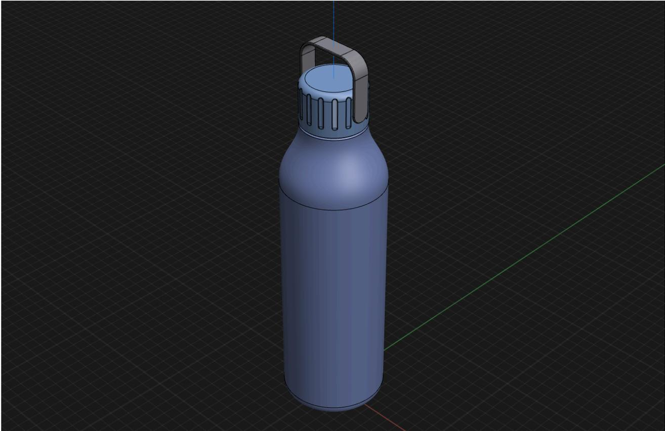
To achieve these grooves, we can use the **Project** tool to project a rectangular-shaped edge onto a cylindrical body and then use the **Chamfer/Fillet** tool to create the desired shape and curves:
