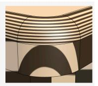
G2 Use this continuity type to create a fillet that matches the curvature of adjacent faces. This produces a smoother transition between the fillet and adjacent faces than G1 continuity. Fillets with G2 continuity will have a non-circular cross-sectional profile.
