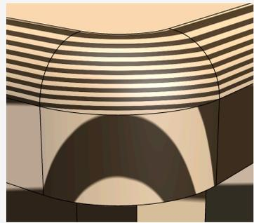
**G2** Use this continuity type to create a fillet that matches the curvature of adjacent faces. This produces a smoother transition between the fillet and adjacent faces than G1 continuity. Fillets with G2 continuity will have a non-circular cross-sectional profile.
