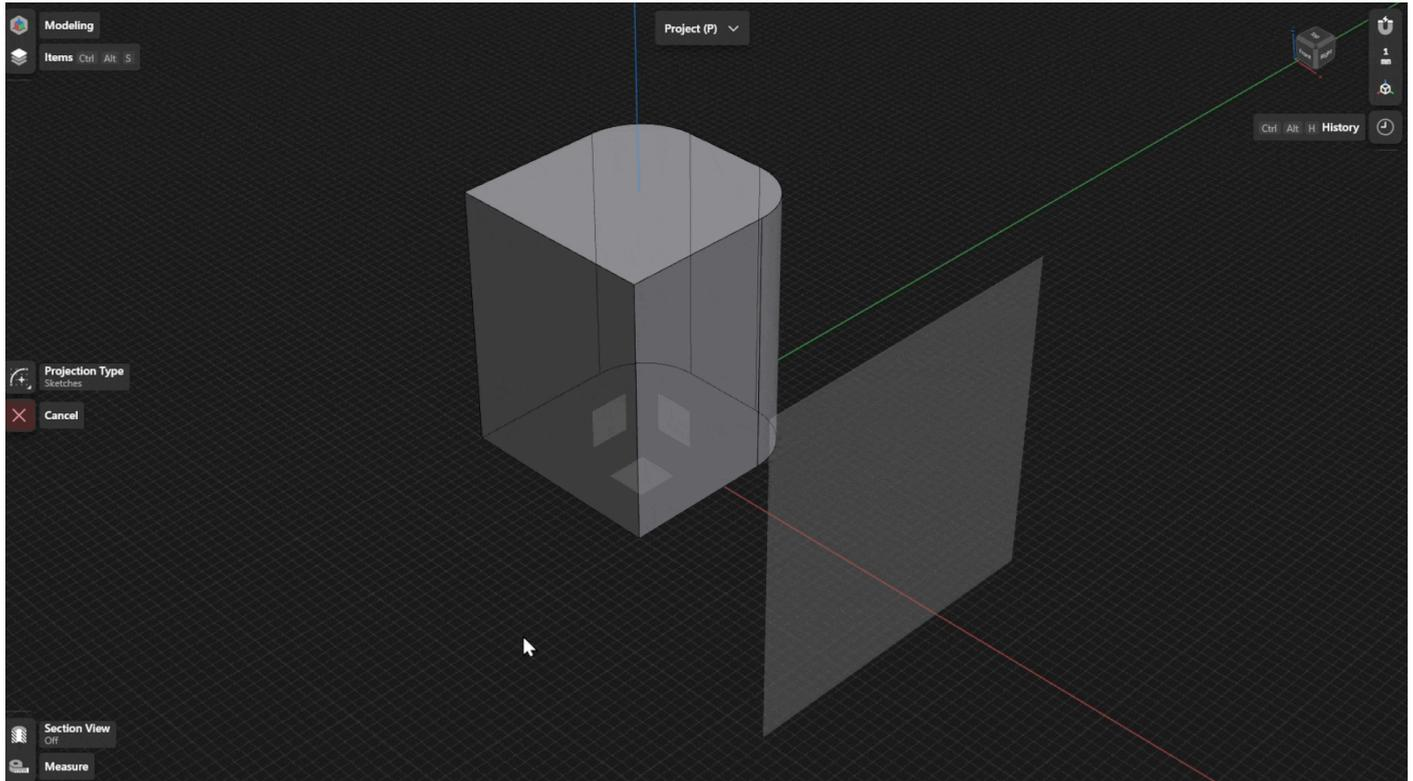
We can then draw the ellipse on the sketch plane while using the sketch projections as guides and then use the [Extrude](#) tool to cut the hole shape we want.
