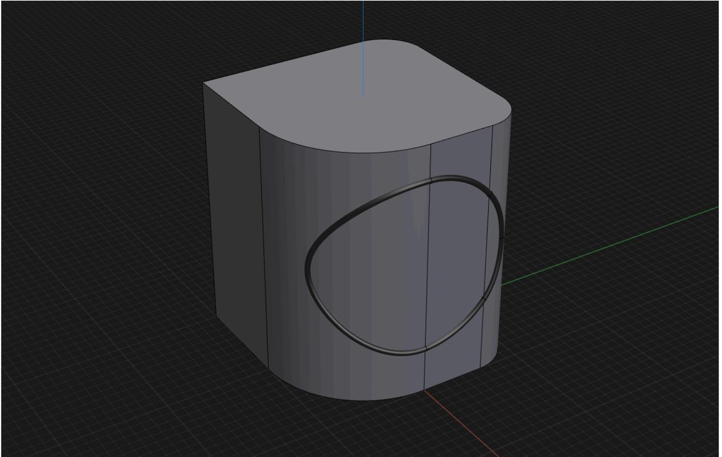
To create this kind of ridge on this particular surface, we can use the **Project** tool to create a circular projection onto the applicable surfaces.
