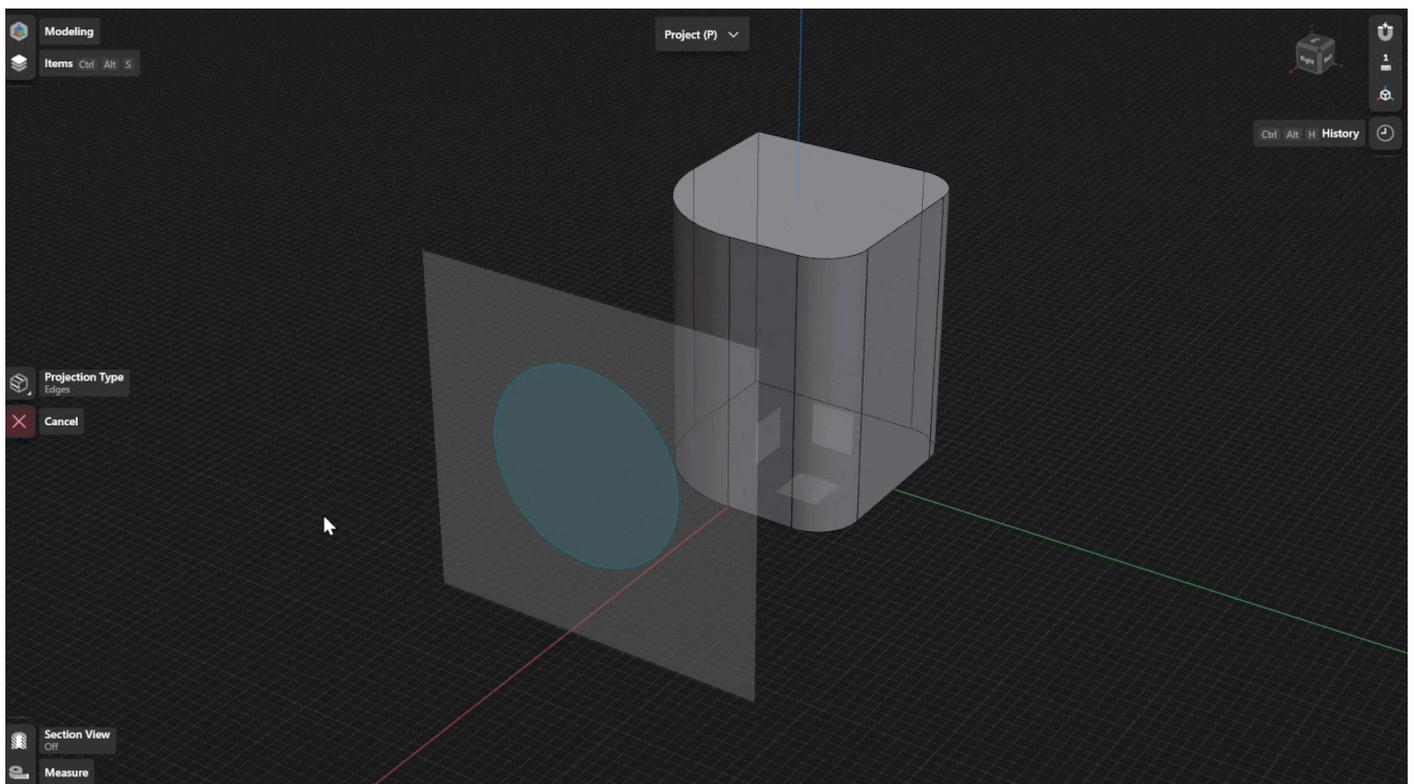
We can then use the [Sweep](#) tool to create the ridge by using the circular projection as the spine or path. To create the sketch profile, we can simply add an [On Curve at Point](#) construction plane to the circular projection.
