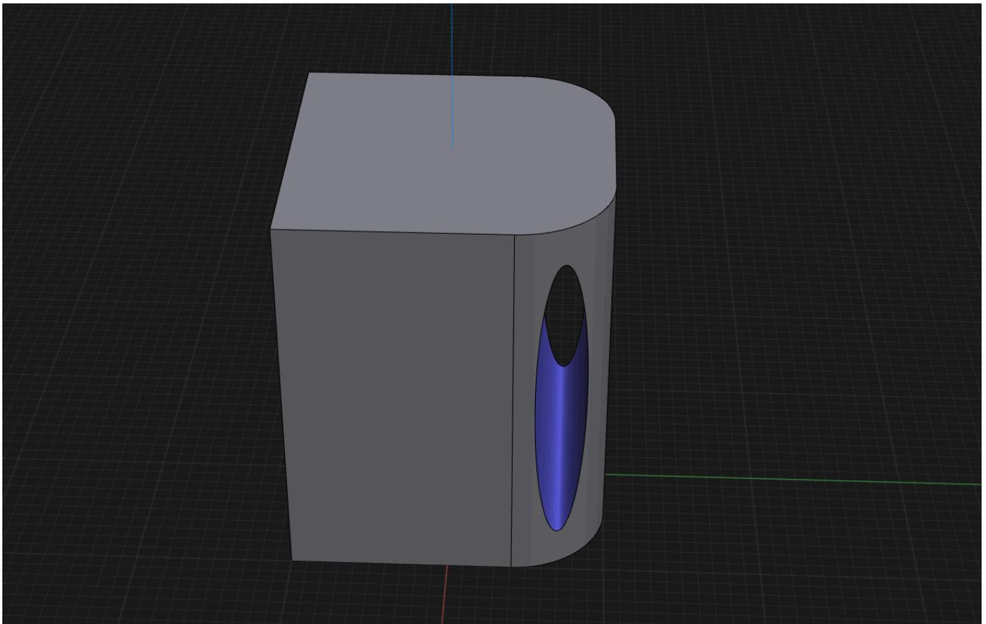
To make a hole that perfectly fits the rounder corners, we can create a sketch projection of the curved edges onto a sketch plane.
